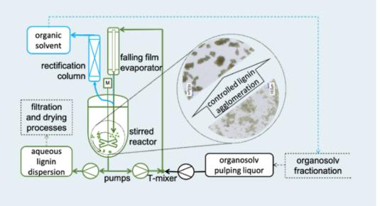
The LigniSep process enables the continuous lignin precipitation from solvent-containing liquors (adapted from Schulze et al., Ind. Eng. Chem. Res. 2019, 58, 3797–3810)
