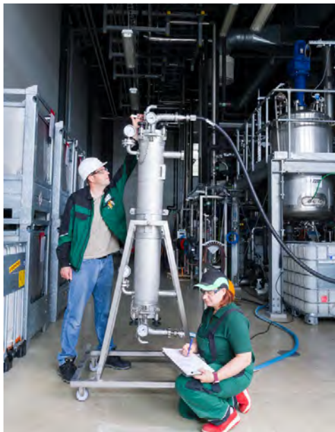
Adsorption column for the purification of liquid mixtures
