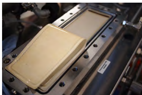
Membrane plant for the separation of liquid mixtures (microfiltration to reverse osmosis)
