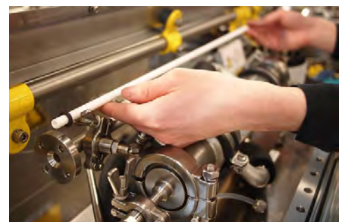
Ceramic membrane for fractionation of solutions in the microfiltration to nanofiltration range
