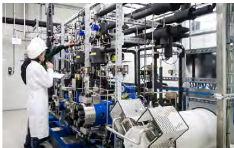
Continuously or discontinuously operating extraction plant, solvents are supercritical \text{CO}_2 (co-solvent ethanol possible) and liquefied propane
