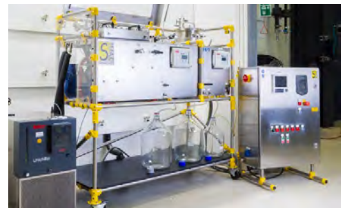
Membrane plant for the separation of liquid mixtures (microfiltration to reverse osmosis)
