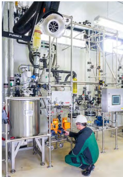
Reaction and distillation plant for the chemical conversion and fractionation of reaction products
