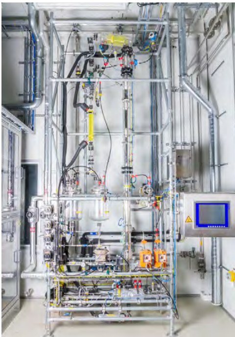
Continuous vacuum rectification plant with up to 100 theoretical separation stages
