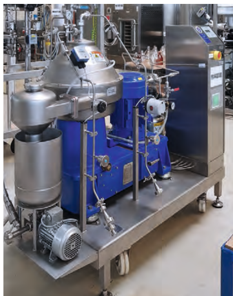
Disc separator for continuous separation of suspensions
