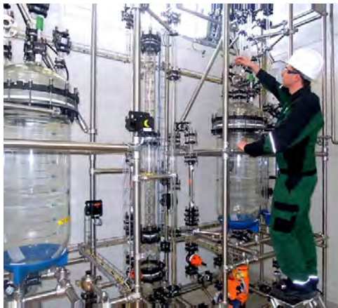
Extraction column with stirrable and heatable product tanks
