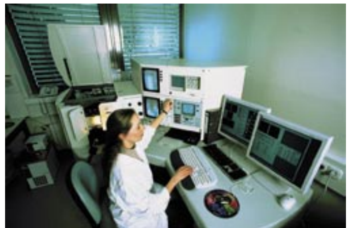
Figure 1: Sorting and separation of specific cell populations from tissues and organs with a FACS-Vantage.
