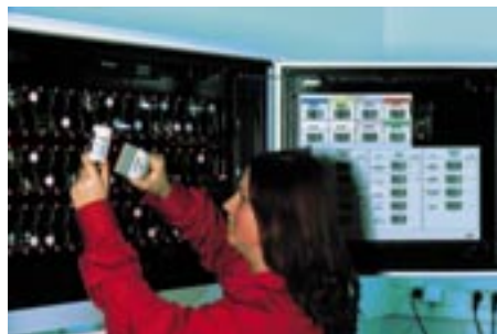
Figure 2: Liquid culture incubator with fluorescence detecting system (Bactec 9120) for automatic sterility testing.
