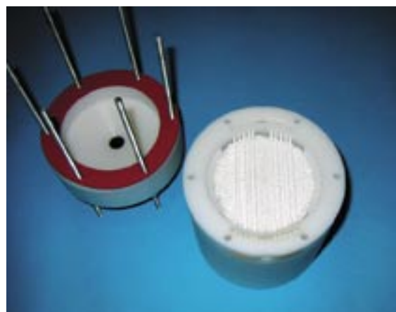
Figure 3: Humidification unit consisting of ceramic tubular membranes and two disks of ceramic foam.
