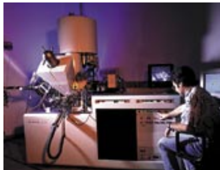
Figure 3: ESCA – electron spectroscopy for chemical analysis – enables the exact determination of the chemical composition of a surface (Kratos, Axis Ultra).
