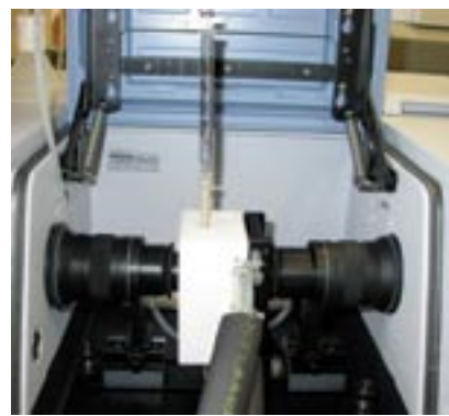
Figure 1: Temperature controlled cell for aqueous protein solutions.
