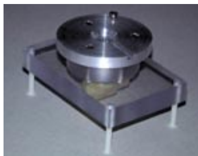
Figure 2: Prototype of a high-voltage cell for physical cell disruption.
