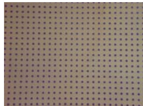
Figure 1: Array of areas, plasma-modified with carboxylic groups ( \varnothing 0.7 mm) and stained with thionine acetate.
