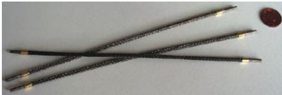
Figure 1: Single capillary fuel cells, which can be assembled as modules.
