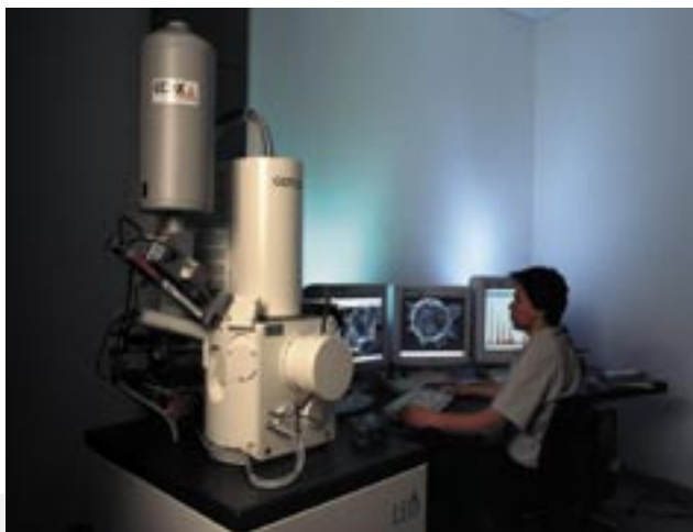
Figure 1: Field emission scanning electron microscope (FE-SEM) with energy dispersive X-ray fluorescence spectroscopy (EDX).
