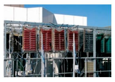
**Figure 3:** Outdoor production plant with ten FPA reactors on the Institute Site in Stuttgart.
