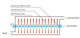
Figure 2: The rotating disk filter developed at the Fraunhofer IGB for use in preliminary filtration as well as in membrane bioreactors.
