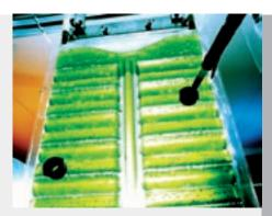
**Figure 3:** Innovative photobioreactor for economic cultivation of microalgae. A controlled flow system provides the algae with optimum light, causing them to grow with a high cell density.
