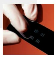
Nanoparticle microarray on silicon chip. Proteins are bound to the nanoparticle via specific linking molecules. The protein chip can thus be used for proteome research or diagnostics, e.g. for the detection of disease-specific antigens or antibodies. The Fraunhofer IGB models and functionalizes diverse nanoparticles and spots them as microstructures onto carriers such as glass or silicon. The chips can then be analyzed with state-of-the art optical screening systems.
