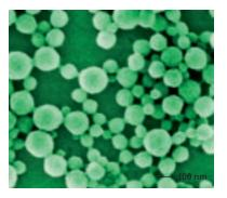
Figure 2: Scanning electron micrograph of molecularly imprinted polymer nanoparticles. Using the lock and key principle, these synthetic particles have the ability to recognize biomolecules.
