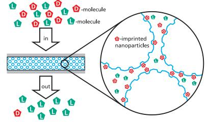
Figure 3: Schematic construction and functioning of a composite membrane with molecularly imprinted polymer particles.
