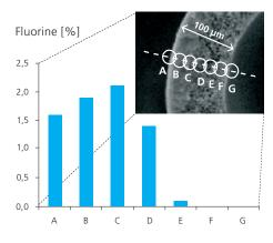
**Figure 3:** Distribution of chemical functionality over the cross section of a hollow fiber following derivatization of the surface-bound amino groups with pentafluorophenylalanine, analysis by ESCA.
