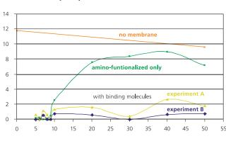
Figure 4: Adsorption of *E. coli* endotoxin (ET) from heparinized blood plasma on hollow fiber membrane modules equipped regioselectively with binding molecules.
