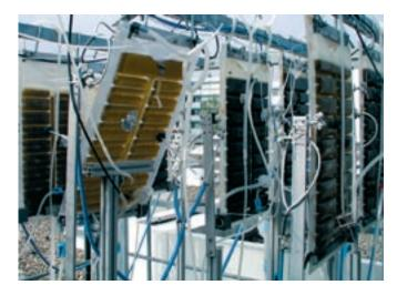
Figure 4: FPA reactors at the outdoor production plant on the Institute Site in Stuttgart.
