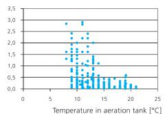
Figure 1: Levels of ammonium nitrogen in the discharge from a treatment plant as a function of the temperature in the aeration tank.
