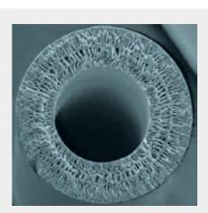
**Figure 2:** Ceramic hollow fibers for microfiltration.
