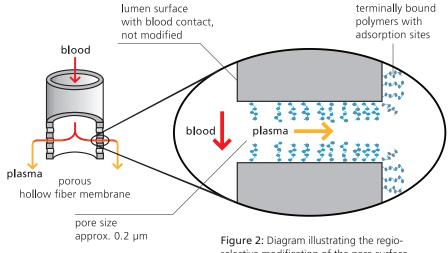
selective modification of the pore surface of hollow fiber membranes by a plasma technique.
