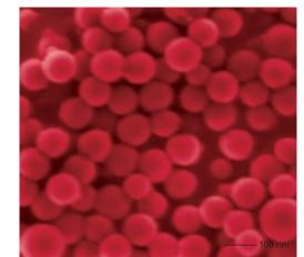
Figure 5: Scanning electron micrograph of biodegradable nanoparticles. These particles can be used for long-term controlled release of active agents in the body.
