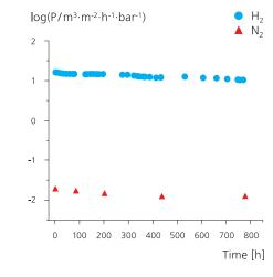
Figure 2: Hydrogen permeability and selectivity of Pdcoated  $Al_2O_3$  capillaries at 430 °C.
