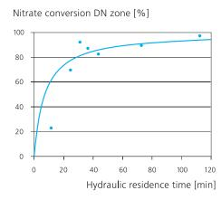
**Figure 2:** Effect of hydraulic residence time on nitrate conversion in the denitrification (DN) zone.
