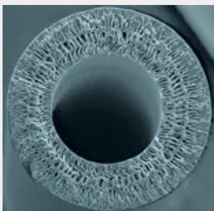
Figure 2: Ceramic hollow fibers for microfiltration.
