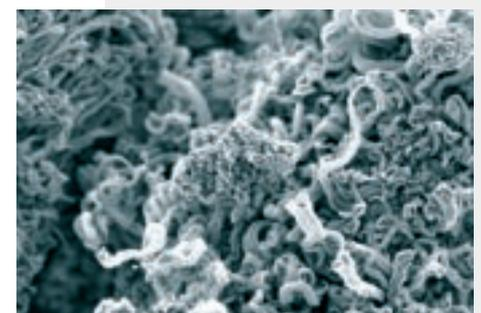
**Figure 2:** Scanning electron microscopy images of different raw materials composed of multi-wall carbon nanotubes (MWNT). The images clearly show the differences in quality in terms of their macroscopic structure.
