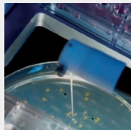
**Figure 3:** A picking robot transfers cells from colonies to agar plates in ordered gene libraries.
