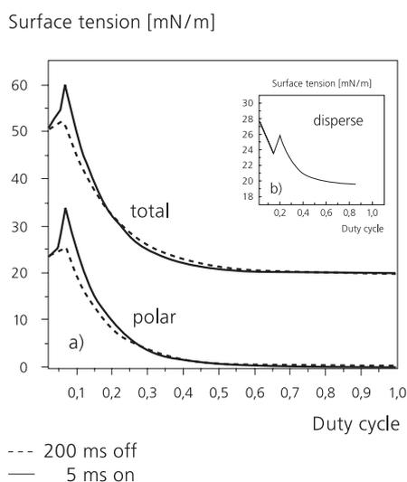
**Figure 1:** The ratio of pulse on time to pulse duration (on time plus off time), referred to as the duty cycle, influences the surface energy of a plasma-treated material. Depicted here is the change in the polar (a) and disperse (b) surface energy components as a function of the duty cycle with constant pulse off time (200 ms) or constant pulse on time (5 ms).
