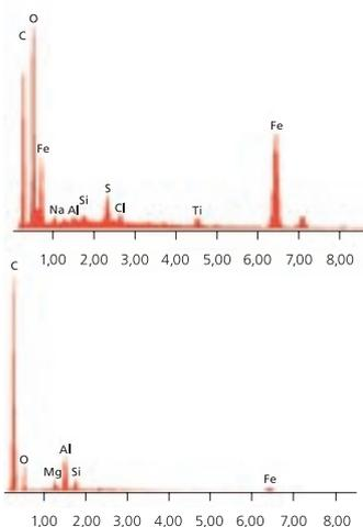
Figure 3: EDX spectra before and after the removal of iron catalysts.
