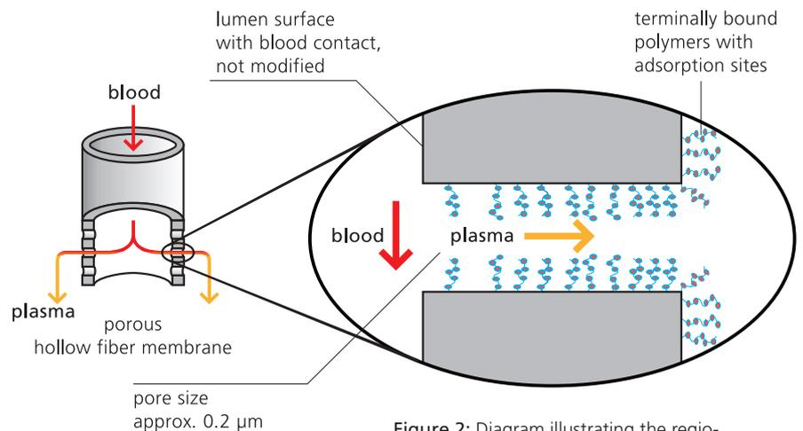
**Figure 2:** Diagram illustrating the regio-selective modification of the pore surface of hollow fiber membranes by a plasma technique.
