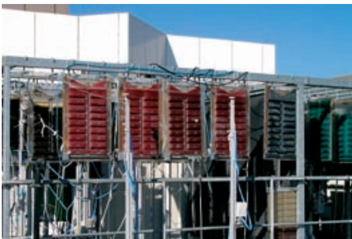
**Figure 3:** Outdoor production plant with ten FPA reactors on the Institute Site in Stuttgart.
