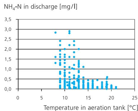
**Figure 1:** Levels of ammonium nitrogen in the discharge from a treatment plant as a function of the temperature in the aeration tank.
