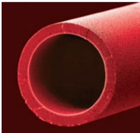
**Figure 1:** The polymeric hollow fiber has an external diameter of 0.4 millimeters. Blood cells flow on the inside, while plasma escapes through its pores and is cleansed of toxins.
