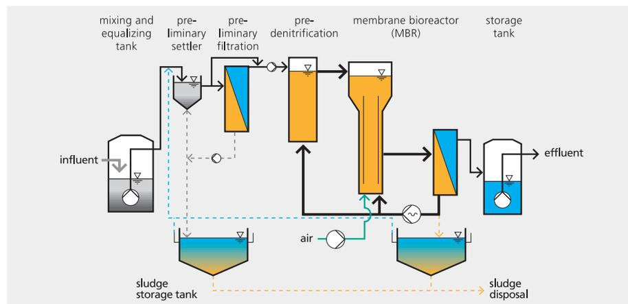
The biological removal of nitrogen is carried out by the process of pre-denitrification. Here, the pre-clarified waste-
