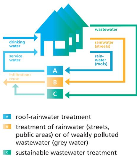
Figure 1: Diagram of water circulation in the new "Am Römerweg" settlement in Knittlingen.
