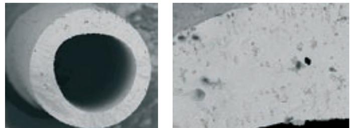
Figure 4 : Typical geometry of a perovskite hollow fiber. Outer diameter 900  $\mu\text{m}$ , inner diameter 600  $\mu\text{m}$ , length 30 cm.
