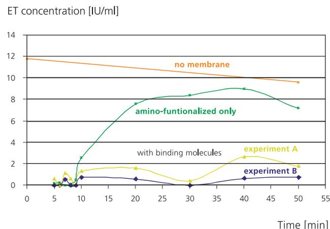
**Figure 4:** Adsorption of *E. coli* endotoxin (ET) from heparinized blood plasma on hollow fiber membrane modules equipped regioselectively with binding molecules.
