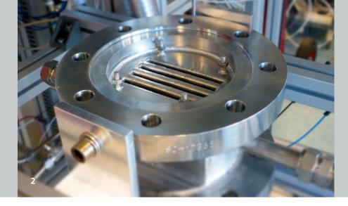
**2** Reactor for producing long-chain alcohols using the Fischer-Tropsch process.
