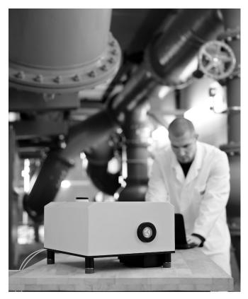
Little larger than a shoebox, the demonstrator was developed as part of the IRLSENS project. It is a quick and automated way to analyze water samples at the waterworks itself. (© Martin Wagenhan/ Fraunhofer IAF) | Picture in color and printing quality: www.fraunhofer.de/press
