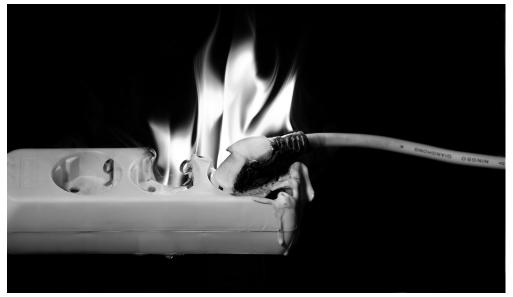
Many multi-plug connectors pose a fire risk, as they can overheat if the current flow is high. Flame retardants in the connector can prevent fires or slow the spread of the blaze. (© Fraunhofer LBF) | Picture in color and printing quality: www.fraunhofer.de/press
