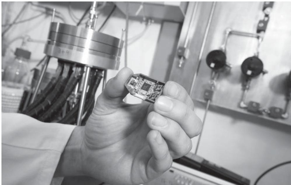
In Fraunhofer IPM's sensor, dyes react to gases – and trigger an alarm, even in the case of smoldering fires. (© K.-U. Wudtke/Fraunhofer IPM) | Picture in color and printing quality: [www.fraunhofer.de/press](http://www.fraunhofer.de/press)
