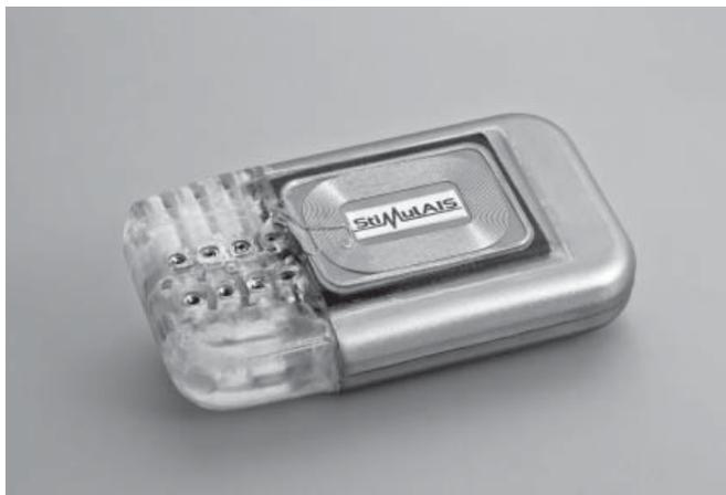
**The implant uses electrical pulses to stimulate muscles. In the future, the unit will be implanted in the patient's groin area. The picture shows the prototype of the implant. (© Fraunhofer IPMS) | Picture in color and printing quality: [www.fraunhofer.de/press](http://www.fraunhofer.de/press)**
