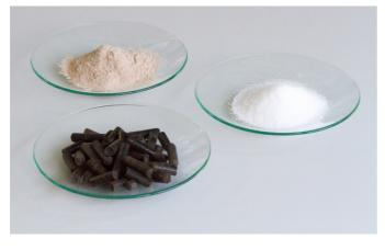
With the BioEcoSim process, livestock manure can be converted into valuable phosphorus fertilizers (rear), nitrogen fertilizers (right) and soil conditioners (front). (© Fraunhofer IGB) | Picture in color and printing quality: www.igb.fraunhofer.de/press
