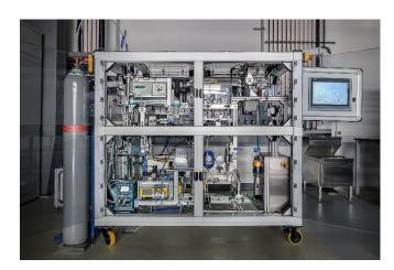
Fig. 2 Lab equipment for cell disruption and extraction of functional materials at Fraunhofer IGB.
