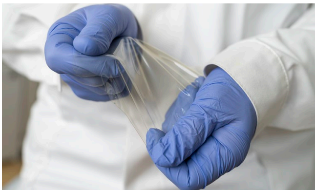
Chitosan films are well suited for packaging applications because of their balanced elasticity and transparency.
