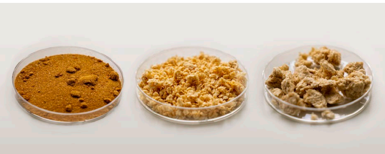
Chitosan (left: derived from A. niger ; middle: from adult flies) and high-purified chitosan from larval exuviae (right)
