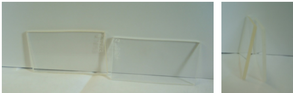
Figure 8: MMA samples made of Itaconic acid sampled from bench scale test. Yellowish MMA was made of itaconic acid from BioConSepT and light MMA with commercial itaconic acid
